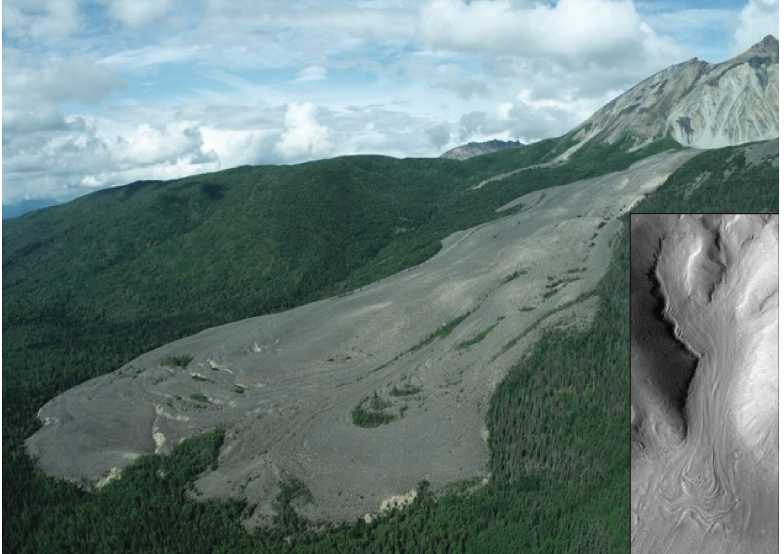
Figure 1.1: Sourdough Rock Glacier (color; acquired via UAV) in Alaska, along with an analogous feature showing ridge and furrow morphology in Deuteronilus Mensae, Mars (black and white inset; cropped from HiRISE image ESP_017130_2255_RED). Both features are approximately 1 km wide at the toe.
